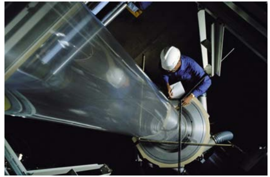
Ongoing temperature measurement of plastics applications such as blown film ensure product quality and productivity. Special models for measuring plastic are available.
