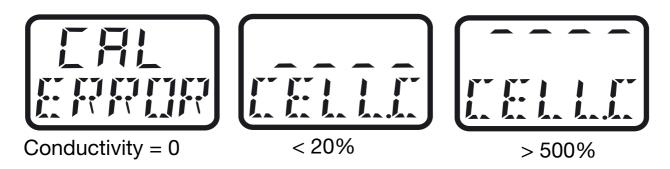
\* The instrument indicates an error.
