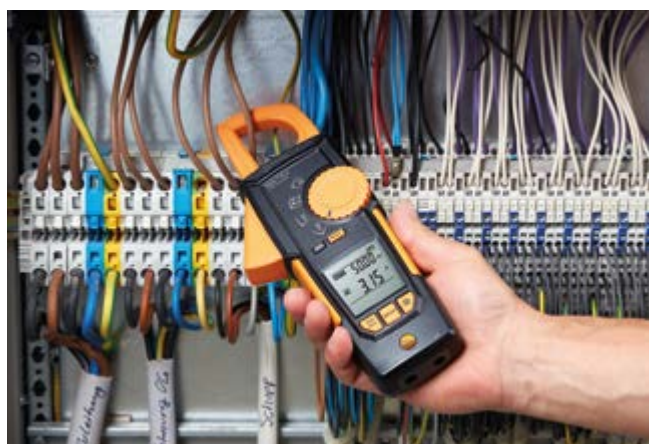
Measuring current in a switching cabinet.
