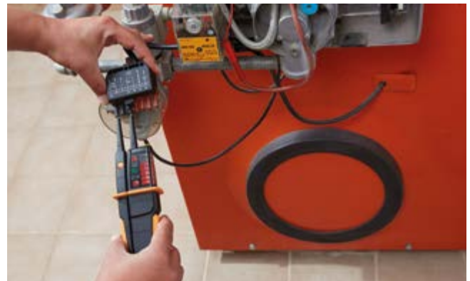
Error detection in a heating system with testo 750 .
