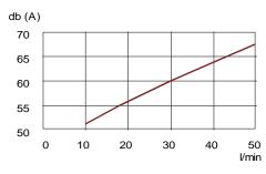
The noise level always remains below the curve with the specified flow value. Test viscosity was 22 mm<sup>2</sup>/s. With a higher viscosity the noise level is lower.
