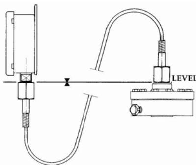
In order to dismantle the instrument more easier for maintenance a shut off valve between the diaphragm seal and the system is recommended (root valve).
