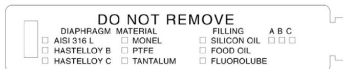
**ATTENTION: Do not remove or slack the filling valve and do not separate the instrument from the diaphragm seal. In case of leakage the assembling is not working anymore and must be returned in order to proceed to a separating circuit refilling.**
