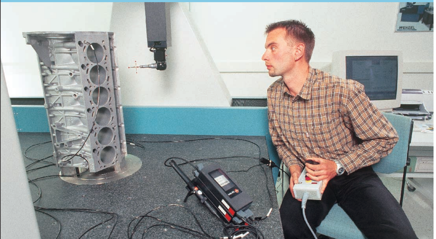
testo 454 Measuring system in use at WENZEL Precision
