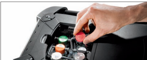
Plug & play: Easy gas sensor replacement
